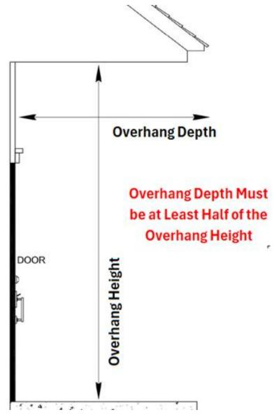
The depth of the overhang must be at least ½ or greater the height of the overhang, or the increased exposure to sunlight and the elements will prematurely wear the finish, seals, frame, hinges, and other hardware.
